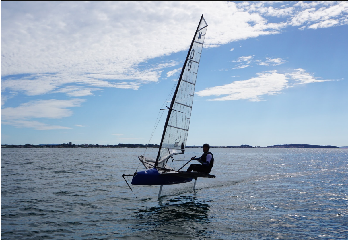
Figure 2.6: Image of an International Moth (Maguire Exocet #4433) sailing in light winds, perfect for showing how the wand mechanism works. The wand touches the water and, through a linkage system ( gearing and offset), it transmits a control input to the foil flap. Image Credit: Luis Sampedro Perez
